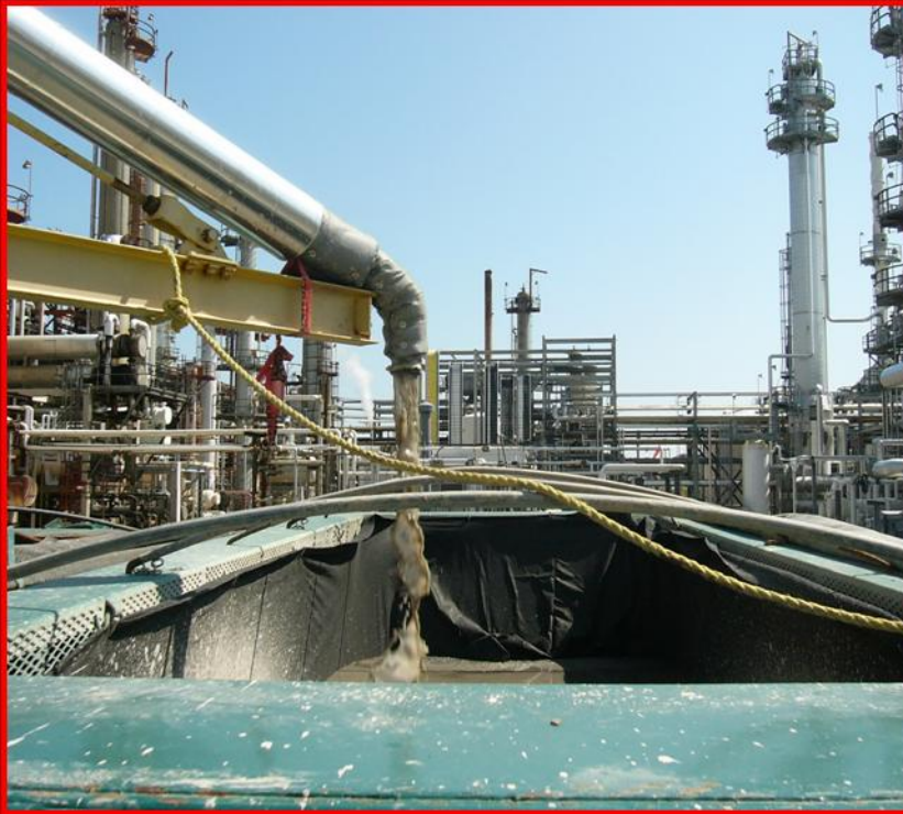
Clarifier Underflow Dumping to Settling Bin
