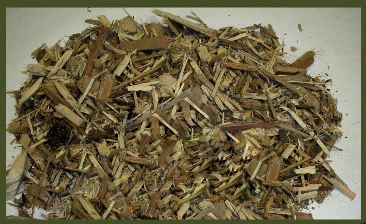
12.9 lbs of previously dried Wood Chips. (Original wet weight of 17.2 lbs At 35% M.C.)
