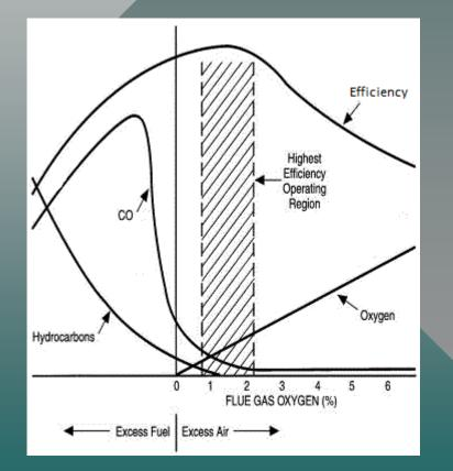
During the load tests, lower excess air until CO begins to rise. Then try to improve mixing to slide the CO and Opacity curves to reduce CO.
