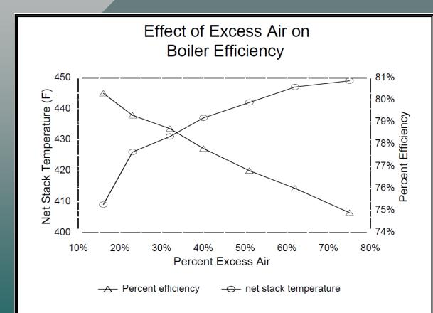
Lowering Excess Air Has a Significant Effect on Stack Temperature
