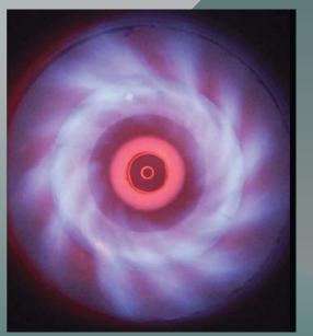
Combustion Air and Flue Gas Fuel Gas Oil Rapid Rapid Mixing Section Furnace Wall Spin or Swirl vane adjustments have traditionally been made primarily by eye, adjusting the mixing pattern by visually observing the flame.
