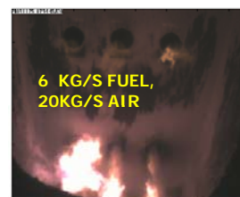
Burner 2-3 appears brightest, but other flames extend beyond image
