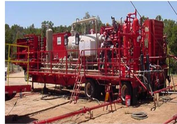
Example of Green Completion Equipment (Source: Weatherford)
