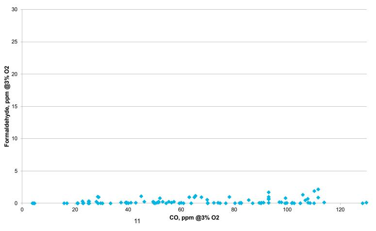
Below 130 ppm @3% O<sub>2</sub>, formaldehyde emissions are consistently low (less than 2 ppm) and trend in a flat line, not downward with decreasing CO emissions.
