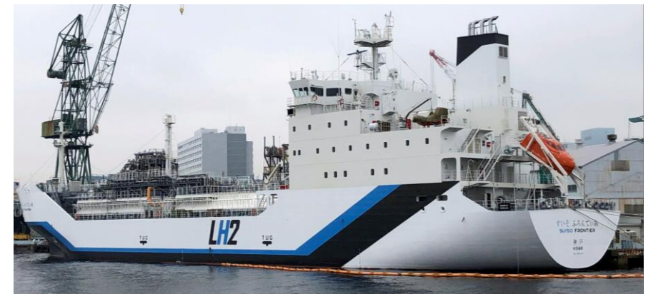
Liquefied hydrogen carrier SUIISO FRONTIER, built by Kawasaki Heavy Industries
