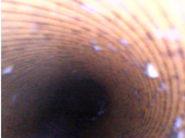
Image 3: Borescope Image of Chiller Tube 1 Year after THERMOPHASE application Without Cleaning in 2022
