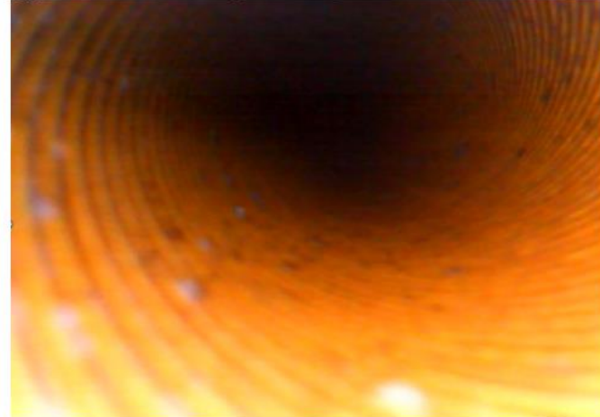
Image 4: Borescope Image of Chiller Tube 1 Year after THERMOPHASE application Without Cleaning in 2023
