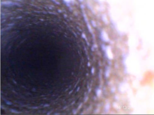
Image 3: Borescope Image of Chiller Tube 1 Year after THERMOPHASE application Without Cleaning in 2022
